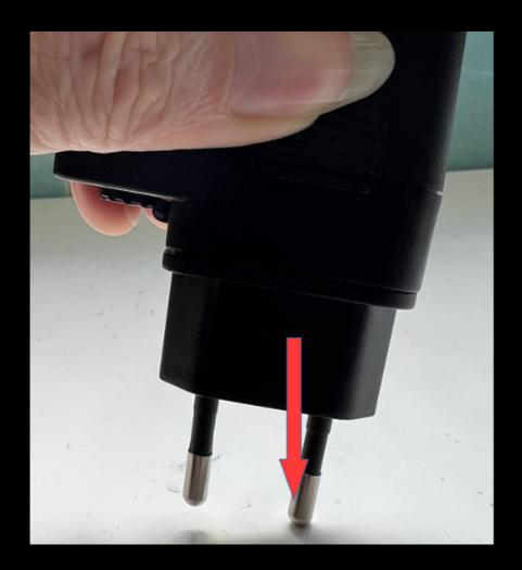
Apply force on the small internal tab by tilting the power supply when pressing down
